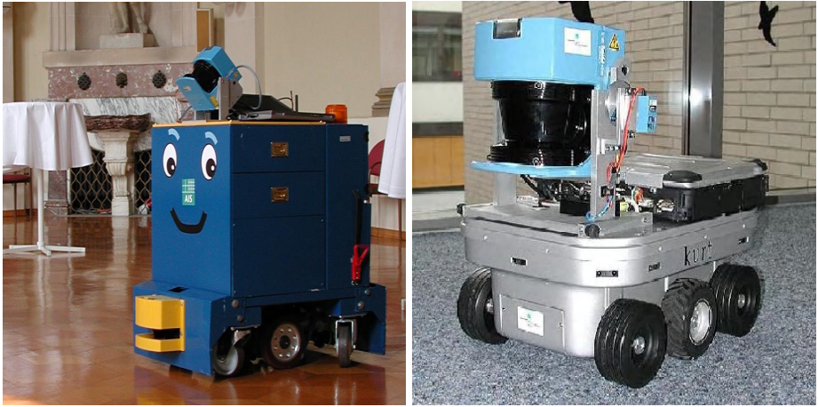
Fig. 3. Left: The Ariadne robot platform. Right: KURT2. Both systems can be equipped with the the AIS 3D laser range finder.
